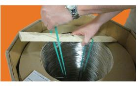
Remove the wood slats and release the rubber bands.
