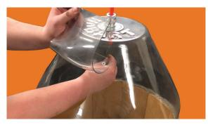
Thread wire into the drum tube. Push wire through the tube into feed roll system. Jog the wire out of the contact tube several feet. Clip and discard the protruding wire.
