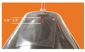
Remove any burrs or flashing at both ends of the Drum Tube (C) and connect to the Drum Tube Connect Kit of Step 1, allowing the Tube to protrude 1/8" - 1/4" below the Connect Kit.
