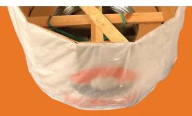
Remove the lid from the drum. Remove the wire tie on the plastic bag and then pull the bag down over the drum.
