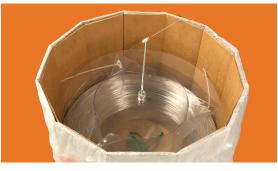
Clip the loop from the end of the wire and insert the Top Hat Spinner device in the drum. Thread the wire into the device.
