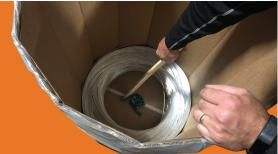
Center the rubber bands in the bottom of the drum so they are not touching the wire. Failure to center the rubber bands in the bottom of the drum can cause wire tangles.
