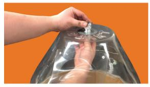
Connect a Drum Tube Connect Kit (B) to the Drum Hood (A). One metal washer should be placed on the inside of the cone, and the other should be placed on the outside of the cone.
