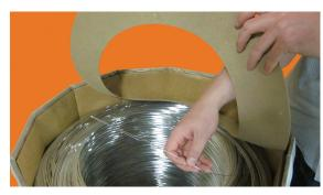
Grasp the end of the wire while removing and discarding the cardboard ring. Pressure should be applied to the wire to prevent it from springing out of the drum.
