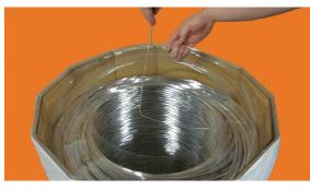
Thread the wire through the inside of the plastic float ring (E) and then rest the float ring on the wire. The apex of the float ring's curvature should point DOWN.
