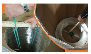
Remove the wood slats and release the rubber bands. Center the rubber bands in the bottom of the drum so they are not touching the wire. **Failure to do so may lead to wire tangles.**
