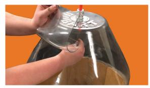
Thread wire into the drum tube. Push wire through the tube into feed roll system. Jog the wire out of the contact tube several feet. Clip and discard the protruding wire.
