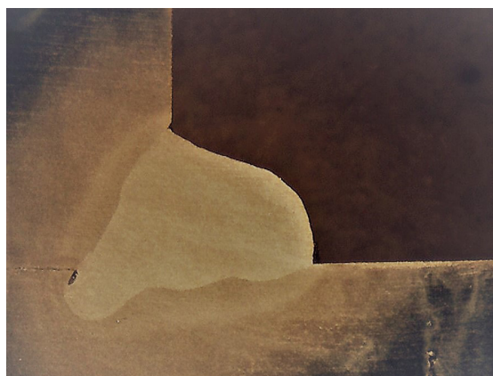
Top Left: Cross-section of a fillet weld made using solid wire at 300 amps
