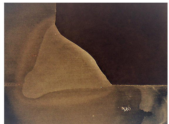
Top Left: Cross-section of a fillet weld made using solid wire at 300 amps
